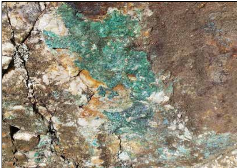
Figure 3-4: Secondary copper mineralisation (malachite \text{Cu}_2\text{CO}_3(\text{OH})_2 ) of fracture coatings overprinting a quartz vein at the Briggs prospect
