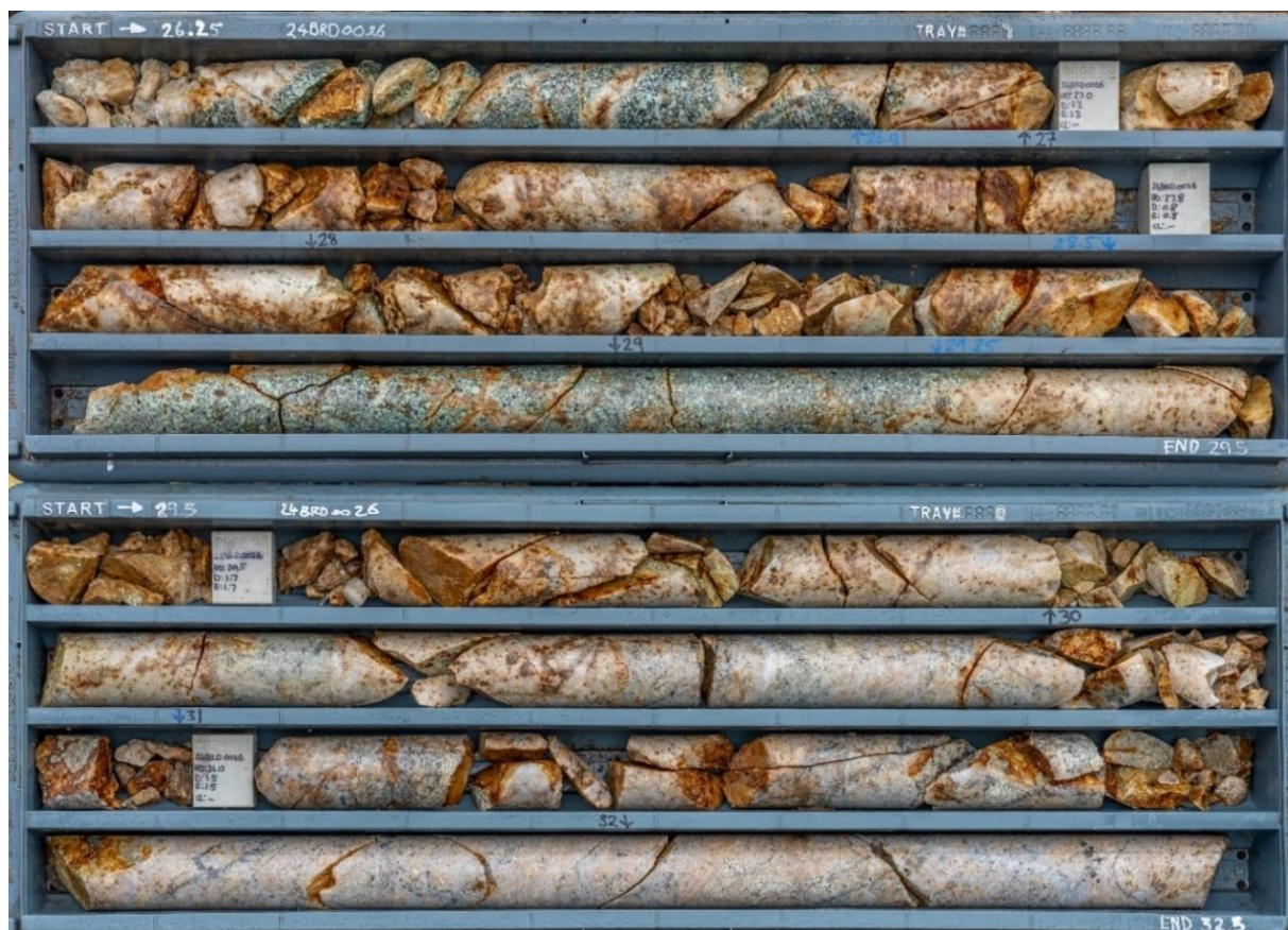
Figure 6 24BRD0026 from 26.25m to 32.5m (av 0.86% Cu). Mineralisation passes from oxide facies (malachite & copper oxides) to a transition zone from 29m where chalcopryite is rimmed by chalcocite and fresh rock from 38m where copper mineralisation is predominantly in the form of chalcopryite for the remainder of the hole.
