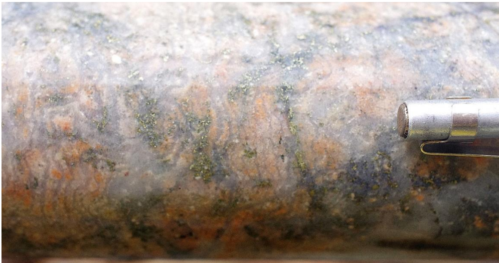
Figure 4 Strongly silicified and altered granodiorite with micro-UST textures and extensive copper sulphides. Hole 24BRD0026 at 40.5m, from a 2m interval which assayed 1.55% Cu.
