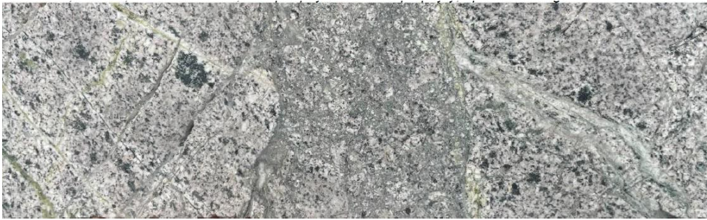
Figure 10 BISM0004 at 166m. Monzodiorite intrusive breccia dyke. Potassic (k-feldspar) alteration. Visually estimated grade of the corresponding sample interval is approximately 0.1% Cu.
