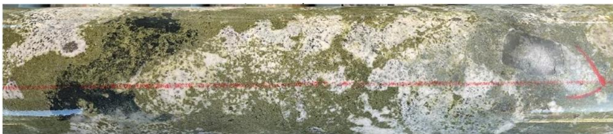
Figure 12 BISM0005 at 133m feldspar (albite?) -epidote-pyroxene (black) skarn alteration. Visually estimated grade of the corresponding sample interval is approximately 0.1% Cu.
