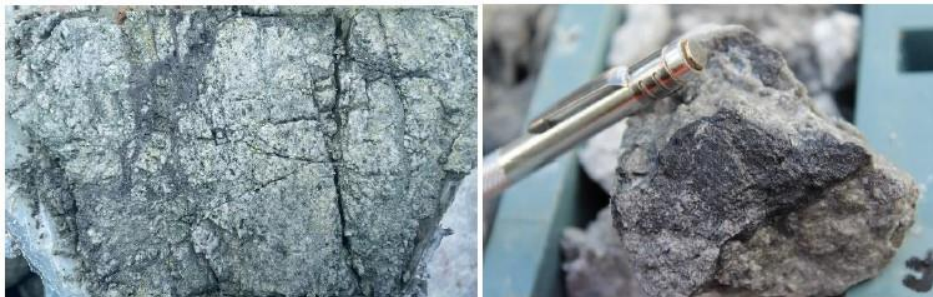
Figure 6 BISM0003 at 150m grey molybdenite as fracture infill. Visually estimated grade of the corresponding sample interval is approximately 500-1000ppm Mo.
